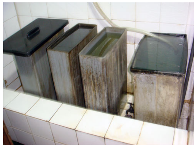
Fig. 1 Wet developing at a non-governmental organisation (NGO) hospital in Port Harcourt, Nigeria demonstrates the need for running water in the rudimentary procedure of developing, rinsing and fixing exposed X-ray films
